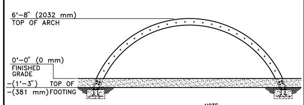
NOTE: CONCRETE FOOTING AND NO. 4 REBAR (BY OTHERS) PER LOCAL SOIL CONDITIONS. CONSULT PROJECT ENGINEER FOR EXACT REQUIREMENTS.
