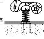
NOTE: CONCRETE FOOTING (BY OTHERS) PER LOCAL CONDITIONS. CONSULT PROJECT ENGINEER FOR EXACT SIZE AND REQUIREMENTS. THREE 5/8" (16 mm) DIAMETER HOLES PROVIDED IN PEDESTAL ASSEMBLY FOR ANCHORING DEVICES (BY OTHERS).
